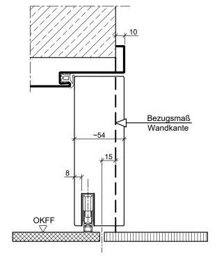
HW54-stumpf in Stahlzarge
